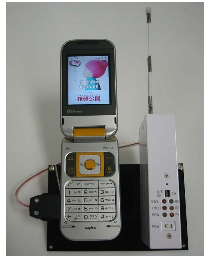
The Activation signal detector connected to a cellular phone
