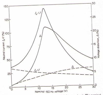
Figure Characteristics of the fluorescent lighting test circuit. The nominal 150 Hz voltage is the calculated product of the 150 Hz lamp current per phase and the circuit zero-sequence impedance (150 Hz). —, Switch S closed (star point to neutral); -----, switch S open (star point floating)
