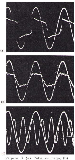
phase current with capacitor one lamp, 240 mA/division; (c) neutral current, three banks of three lamps in star,240mA/division
