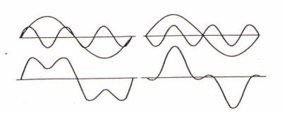
FIG. 1 Effect of harmonic phase angle on waveshape.
