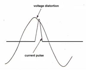
FIG.2 Current pulse from television reciever with thyristor power supply and consequent voltage distortion
