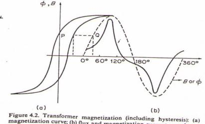
magnetization curve; (b) flux and magnetization current waveforms
