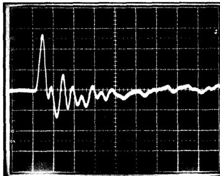
Figure 2. Impulse response of badly braced cabinet.
