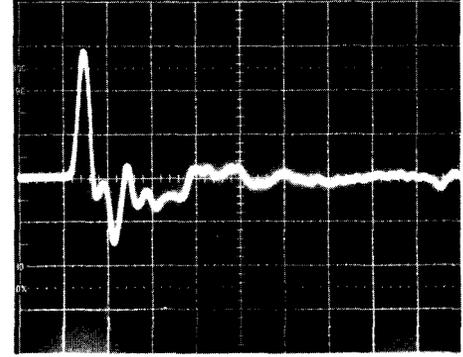
solving the enclosure ringing problem. Bear in mind, though, that if a surface can move it will resonate at certain frequencies. Constructing a properly braced cabinet usually reduces this problem significantly. Ultra Sound has researched the ringing problem with Hard Truckers Speakers, of San Rafael, California, to improve enclosure construction and bracing.
