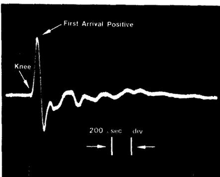
Figure 1. Typical impulse received at microphone. Horizontal scale = 200 microsecond/div.
