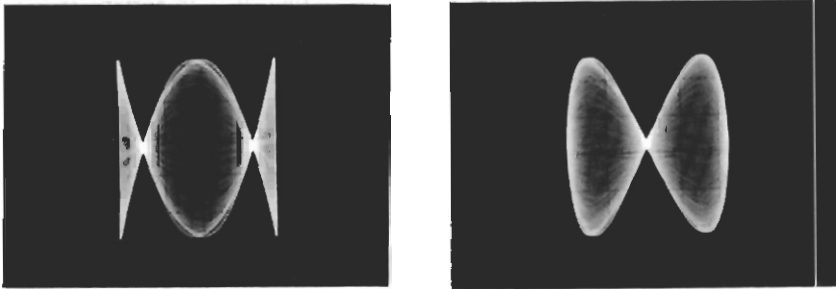
Fig. 2-2 Subcarrier and pilot signal phasing.
