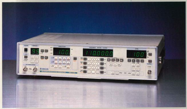
The JSG-1100B is a versatile instrument, specially developed and designed to generate FM and AM signals as well as FM stereo signals used in the radio production line. The carrier frequency range covers 100 kHz to 110MHz and the FM stereo band, 75 to 110 MHz. PLL system is employed for high accuracy and stability in generation of the carrier frequencies. All operating functions are microprocessor-controlled and set values are displayed digitally.
