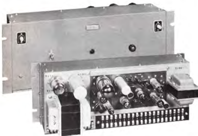
Fully regulated power supply. Relays are powered from main power supply and located inside of drop-panel housing.
