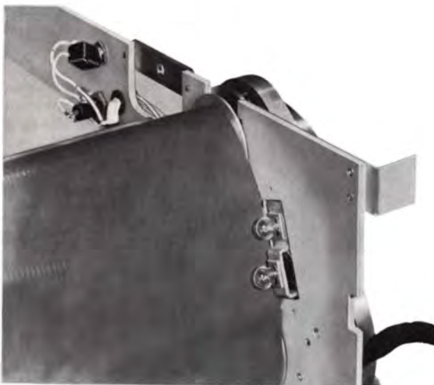
Through transparent slits in tape, special lamps and photocell arrangement control stop, cue and rewind of tape.
