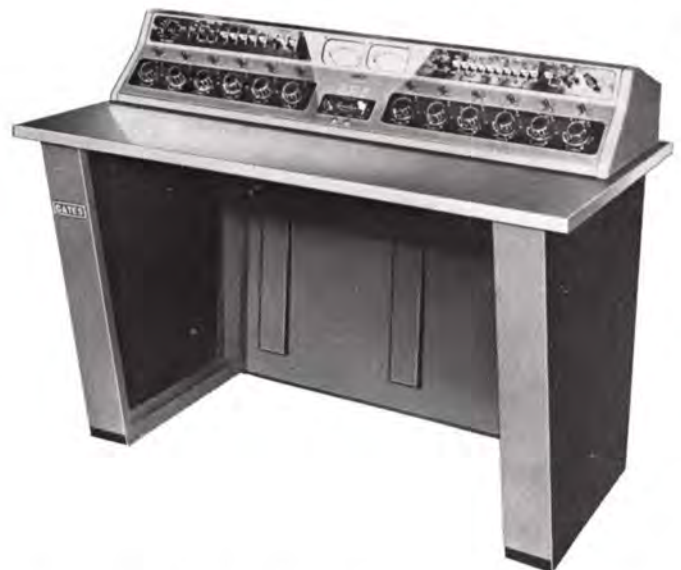
Dualux and desk. Desk designed specifically for the Dualux, with sides and back of 16 gg. stretcher level furniture steel finished in medium gray. Top is of formed linen formica in charcoal gray attached to seasoned 5-ply birch. Three wiring troughs extend down the inside rear to conceal wiring from console to floor. Leveling screws are on all four corners. Size: 47" wide, 30" front to back, height 29" adjustable to 30 1/4". Shipped knocked down.
