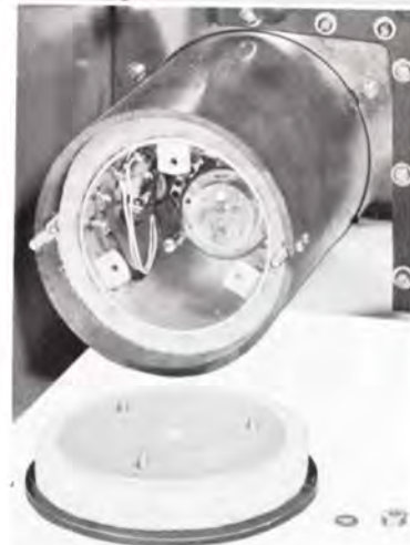
Above is the crystal oscillator unit, heart of the M-4990 frequency monitor. The open view illustrates the vacuum crystal, under which are the oscillator components, all temperature controlled. The oscillator tube, however, is external to the temperature chamber. The entire unit is plug-in and there are no variable air gaps for frequency adjustment at time of installation.
