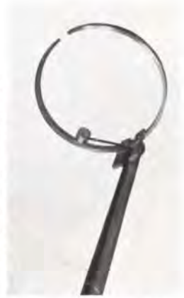
Two ring antenna, power gain of 1.3 .. Type FM-22 Broad band antenna ..... Type FM-11
