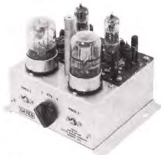
⏏ Dual vacuum mounted crystals are designed into a new oscillator with the emphasis on stability and dependability. ⏏
