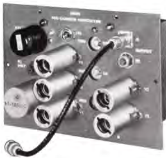
Front and rear view of sub-carrier generator. Illustration on previous page shows one sub-carrier generator installed on the sub-inserter panel with space for second sub-carrier generator provided. Sub-carrier generators are identical other than frequency of operation.
