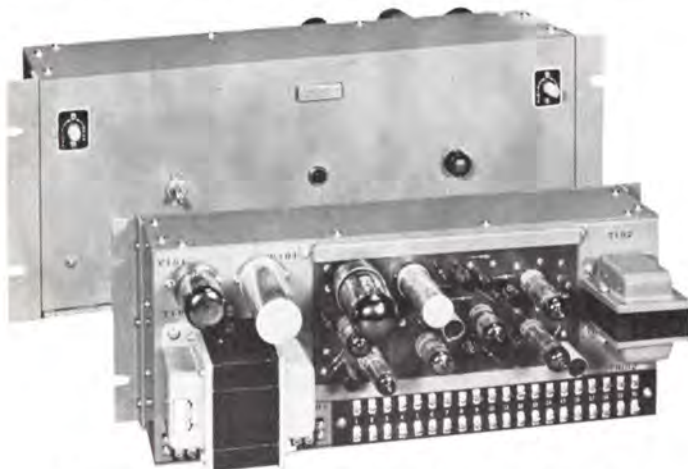
Power supply and monitoring unit; drop-panel housing.
