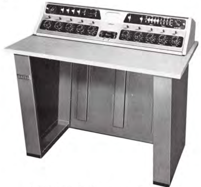
Desk designed for Gatesway console. Sides and back of 16 gg. stretcher level furniture steel finished in medium gray. Top is of formed linen formica in charcoal gray attached to seasoned 5-ply birch. Three wiring troughs extend down the inside rear to conceal wiring from console to floor. Leveling screws are on all four corners. Size: 39 \frac{1}{2} " wide, 30" front to back, height 29" adjustable to 30 \frac{1}{4} ". Shipped knocked down.
