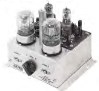
Open and closed views of the new ovenless, low drift crystal oscillator — first IPA unit.
