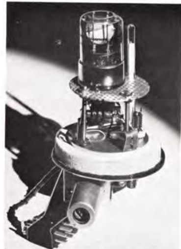
Rear view of M-4990 frequency monitor with dust cover removed. Each resistor and capacitor is firmly secured to the printed wiring chassis. Parts stacking is obviously absent.
