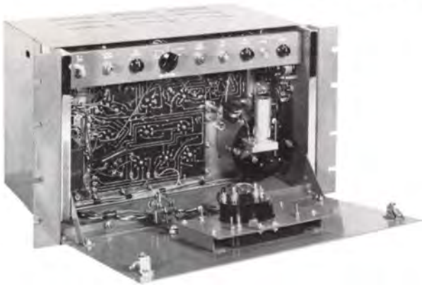
Front panel hinges down to expose operating adjustments and the plug-in crystal unit. Here is exhibited the uniformity of printed wiring to produce uniformity in year-in and year-out service.
