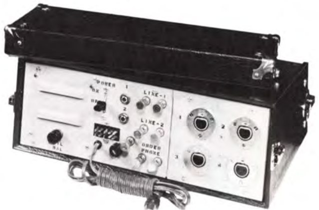
Back of the Dynamote handles all connections, microphones and even holds the Off-On switch. Receptacle in center is for accommodating the optional M-4933 battery unit.
