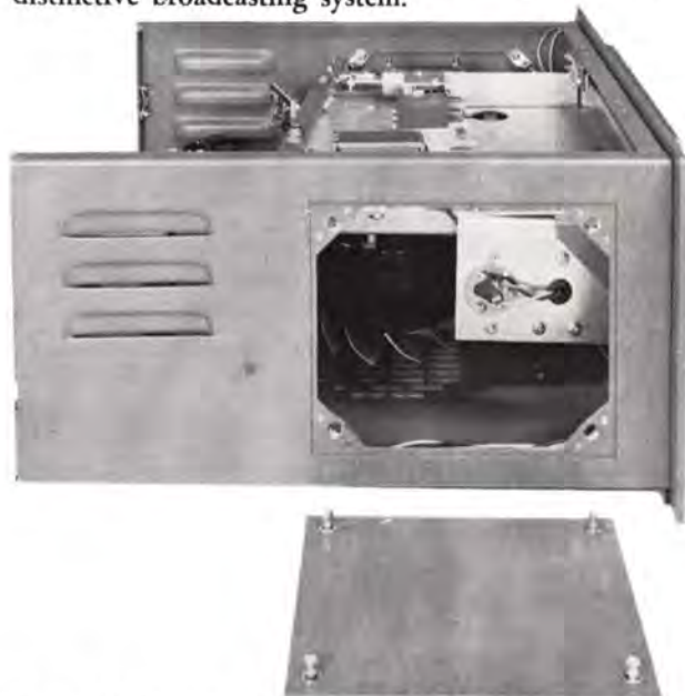
The Gates Carritape offers complete accessibility for maintenance. Each side slips off with quick fastener screws.
