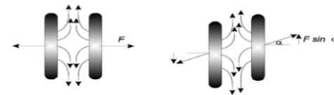
working principle of the magnetic anti-spring system. When the magnets are displaced in the vertical direction (right side) a vertical component of the repulsive force appears.
