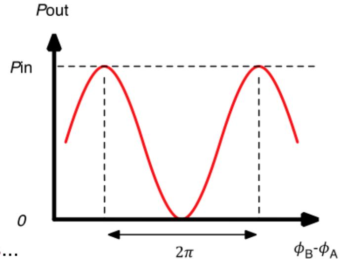
The max response to  $h$  is at  $\pi/2$  but **laser power fluctuations...**
