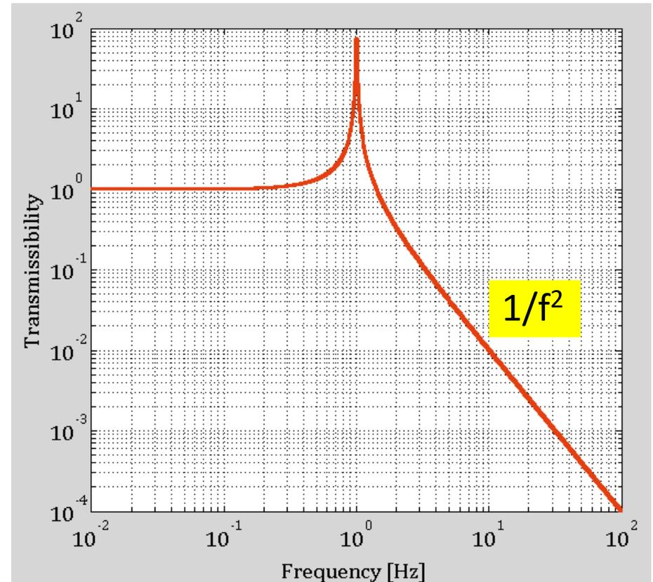
The suspension also provides attenuation of ground vibrations, ... but far from the  $10^8$ - $10^{10}$  seismic attenuation required in the GW detection band (10 Hz - 3 kHz)
