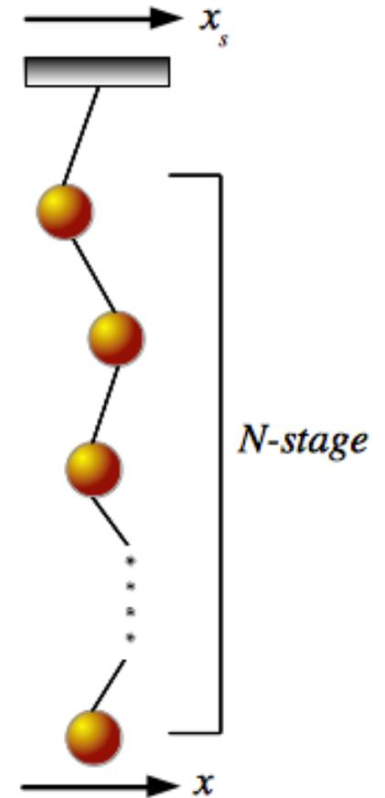
Above the seismic isolator cut-off the mirror responds as a single simple pendulum
