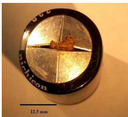
Fig. 10. Field-failed capacitor showing venting.
