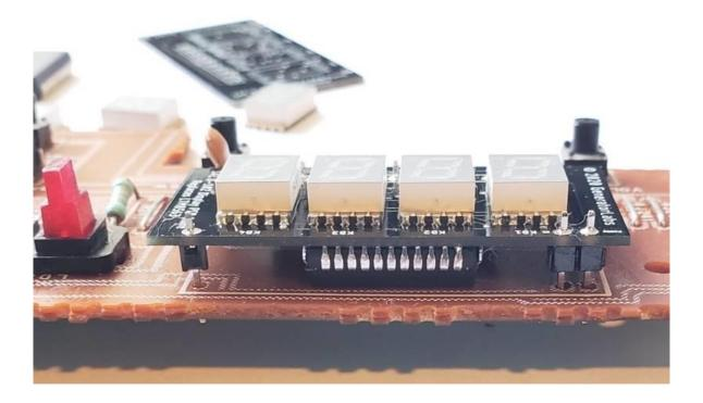
Also notice the 4 seven segment LED's. Those are surface mount devices and they also add to the thickness of the entire device. Be very careful when placing the internal bezel over the newly installed assembly. It is very old plastic and tends to get brittle. If you force the bezel to do something it does not like it may crack. Do not say I didn't warn you!
