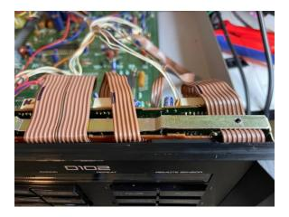
The style of ribbon cables in the D102 are far from ideal. Pay close attention to the individual conductors. The flimsy wires can jump positions, can bend and not fully seat or 2 wires could inadvertently occupy one slot in the header. Again, this can have disastrous results. <u>You must inspect closely!</u> Two wires occupying the same slot is very easy to miss!
