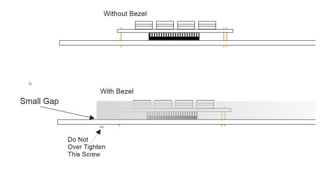
**IMPORTANT!** The screws that hold the metal top cover on are different lengths!!!! Make sure the screw that is in the middle of the cover, just above the LED display is the shortest screw. If you put a long screw in that position it will push the LED digits downward, making them appear misaligned. It could also cause permanent damage or a short-circuit. All of the cover screws may appear short but some are purposely shorter than others.
