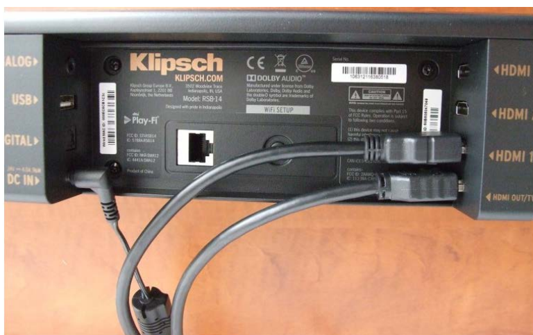
Note that the HDMI 2.0 connectors are compatible with HDCP 2.2. As such, they handle 4K UHD video stream, which they convey without processing (Passthrough) from the source to the display.
