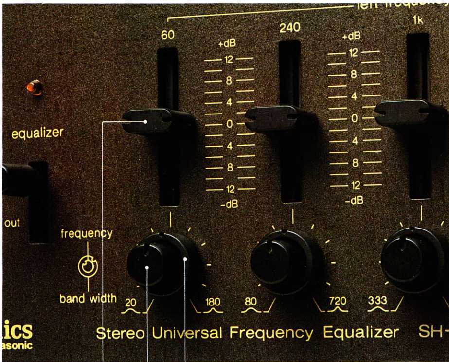
Slide Pot Bandwidth (Q) Control Center Frequency Control
