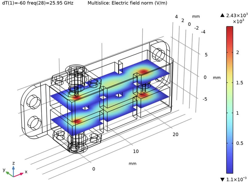
*Figure 6: Electric field norm around the center frequency of the EU millimeter-wave 5G band when the temperature is  $-40^\circ\text{C}$ . The thermal-structural deformation did not distort the dominant TE resonant modes in the cavities.*
