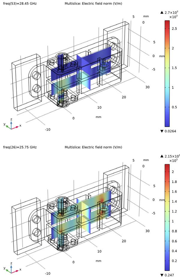
*Figure 9: The electric field norm beyond the passband is presented at the top, with the input signal failing to reach the output port. Conversely, the electric field emanating from the excited port was detected with minimal attenuation at the center of the passband, as illustrated at the bottom.*
