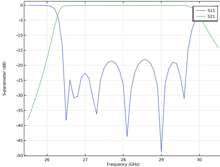
Figure 3: S-parameter plot for the millimeter-wave 5G band for Japan, Korea, and the US.
