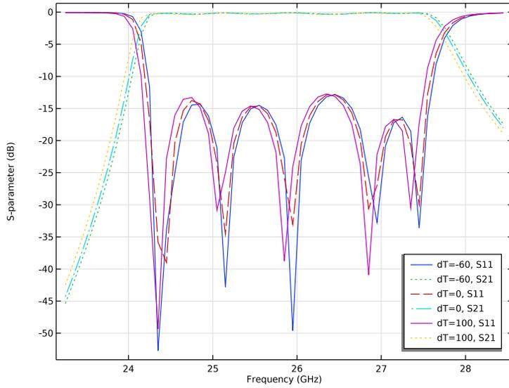
Figure 7: S-parameters are slightly shifted as a function of ambient temperature.
