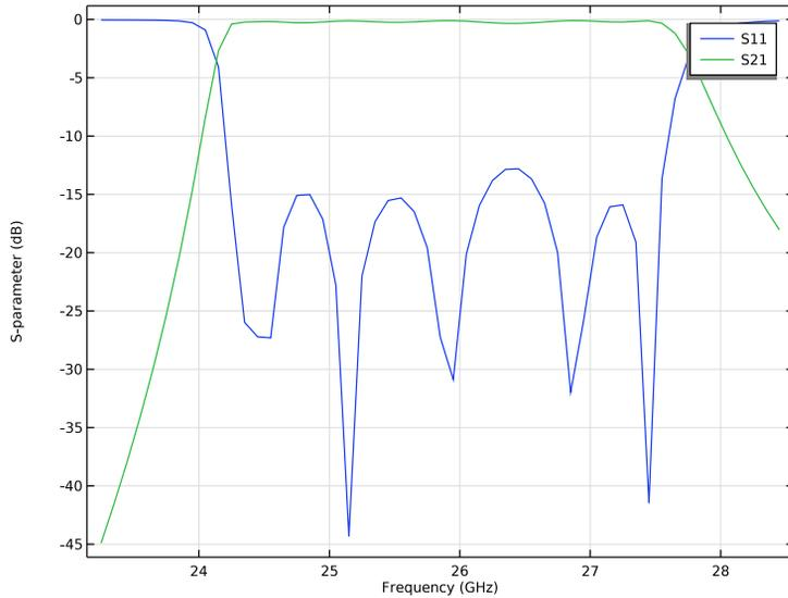
Figure 5: S-parameter plot for the millimeter-wave 5G band for EU and China.
