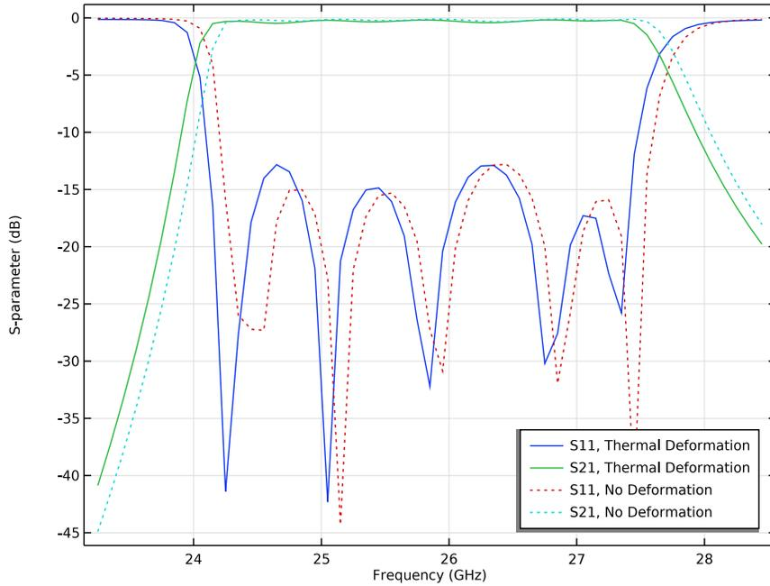
*Figure 10: S-parameters affected by the uneven heat source from the baseplate.*
