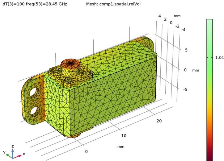
Figure 8: Thermal expansion at 120°C that is 100K above the reference temperature.
