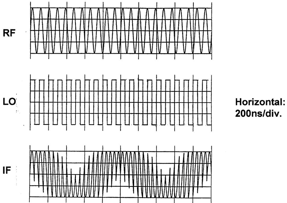
**Figure 4.5:** Inputs and Output for an Ideal Switching Mixer
