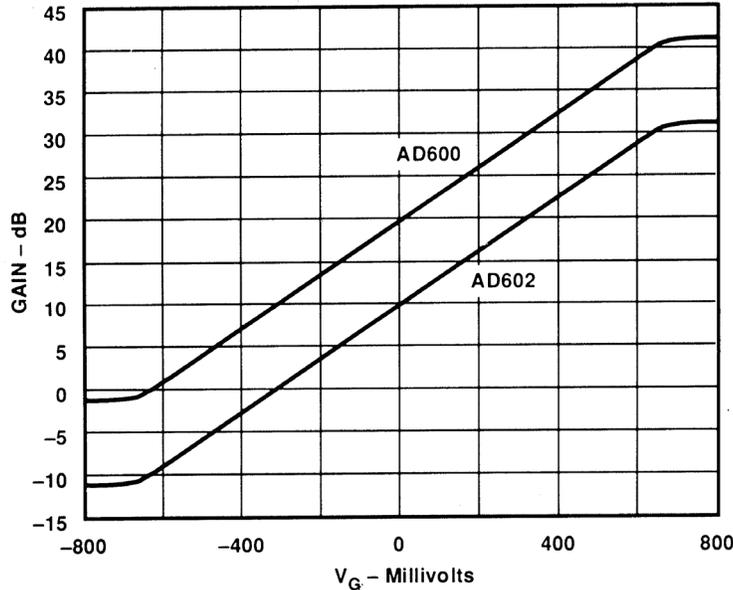
**Figure 4.35:** X-AMP Transfer Function
