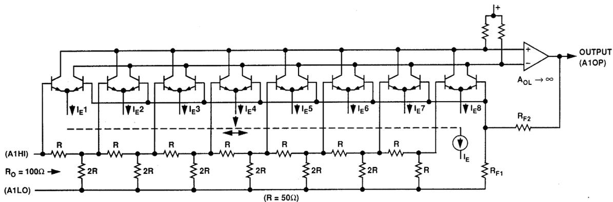
**Figure 4.36:** X-AMP Schematic
