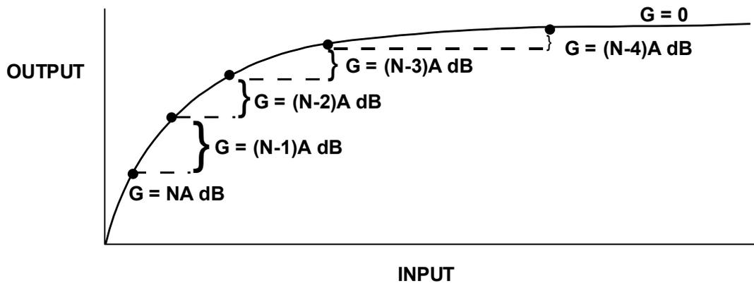
**Figure 4.21:** Basic Multistage Log Amp Response (Unipolar Case)
