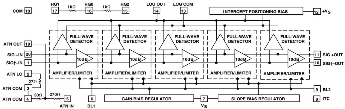
**Figure 4.25:** Block Diagram of the AD641 Monolithic Log Amp
