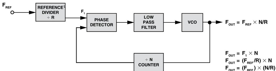
**Figure 4.56:** Using a reference counter in a PLL synthesizer.
