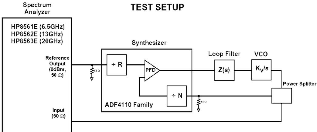
**Figure 4.66:** Measuring Phase Noise with a Spectrum Analyzer
