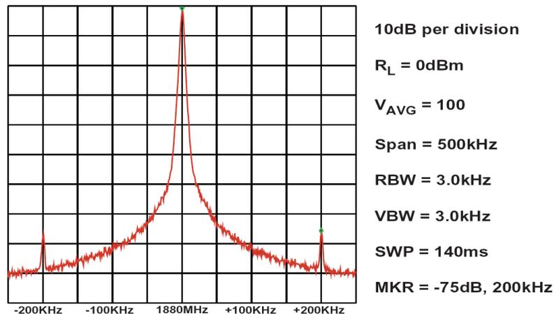
**Figure 4.70:** Output Spectrum Showing Reference Spurs.
