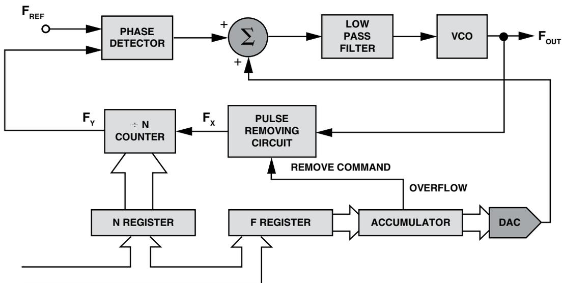
**Figure 4.59: Fractional-N Synthesizer**
